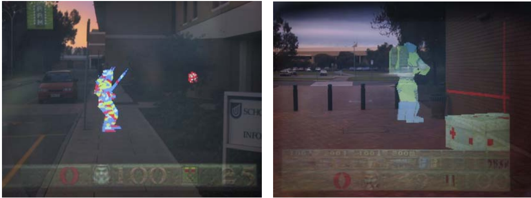
Figure A-15 ARQuake implemented using optical AR with virtual monsters shown
