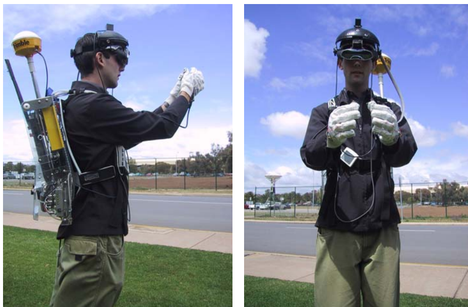
Figure A-21 Side and front views of the Tinmith-Endeavour backpack in use outdoors
