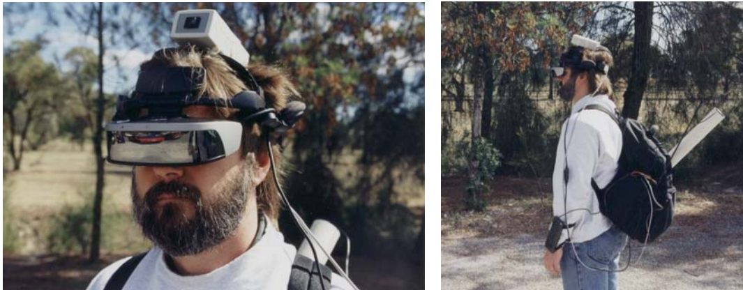
Figure A-2 Map-in-the-Hat prototype inside ruck sack, with antenna, cables, and HMD
