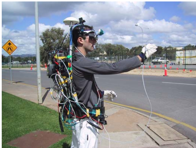
Figure A-17 Side view of original Tinmith-evo5 backpack, with cabling problems
