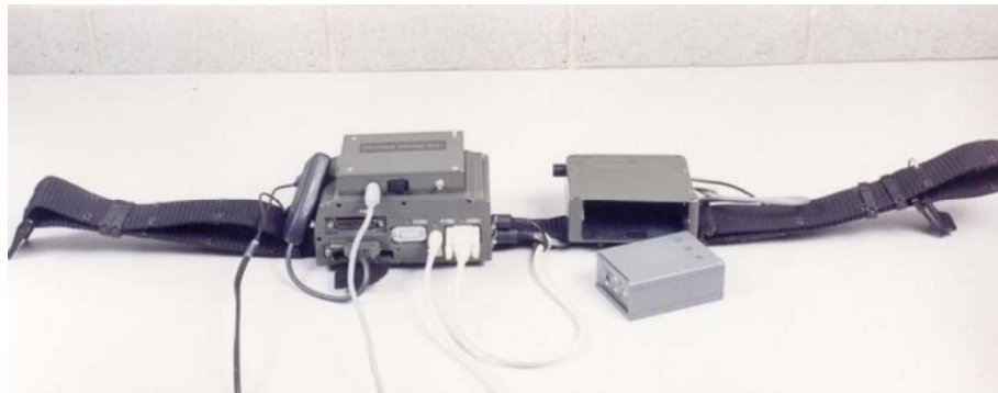
Figure A-1 Phoenix-II wearable computer with batteries, cables, and belt mounting
